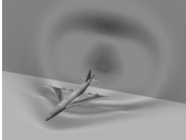
Figure 11: Pressure Contours and Sonic Boom on a Representative HSCT Configuration
